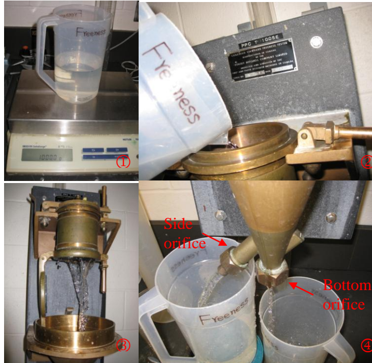
Figure 12: Sequence of using Freeness beakers to carry out calibration. 1: Weigh 1000 g of 20 °C distilled water; 2: Pour the water into the chamber; 3: Open the valve and bottom lid to release water; 4: Receiving water from side orifice.
