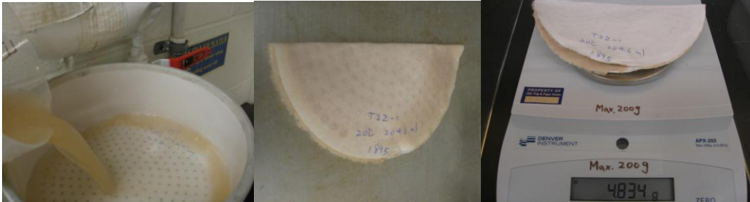
Figure 15: On the left, suspension is being poured to Buchner funnel with a tared filter paper; on the middle, pad is dried in a speed dryer; on the right, check the OD weight of pad.
