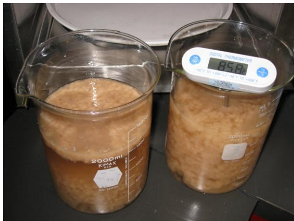
Figure 6: The suspension has been heated and is at ~85-90°C.
