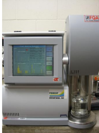
Figure 26: FQA, Fiber Quality Analyzer with a 600-ml sample beaker.
