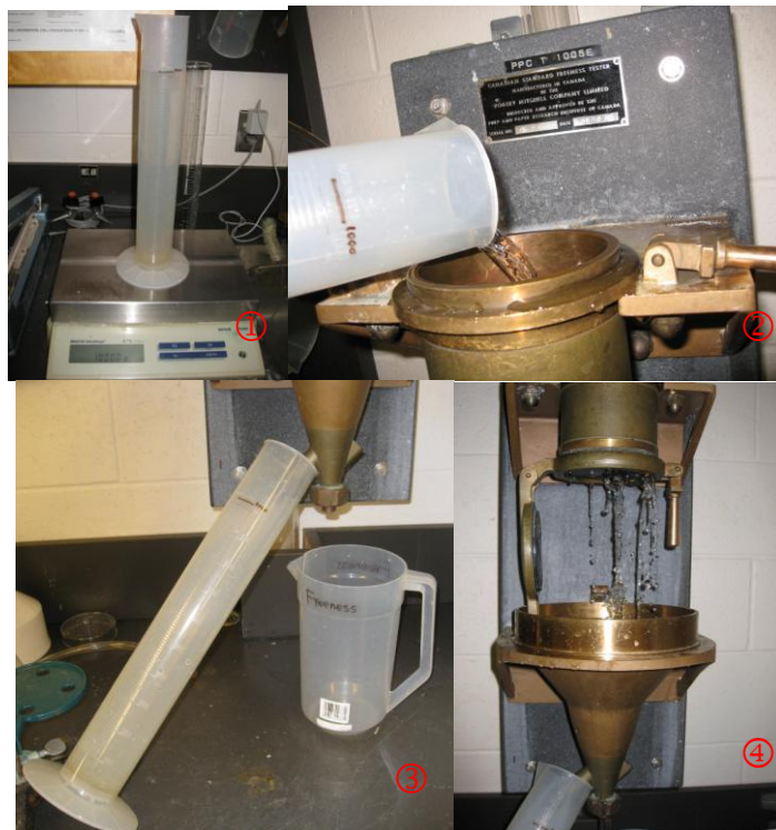
Figure 13: Sequence of using 1000 mL graduated cylinder to carry out calibration.
