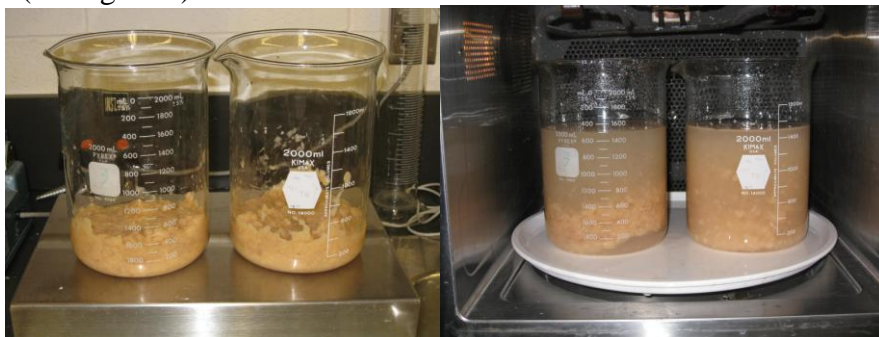
Figure 5: On the left, weigh pulp slurry in beakers; on the right, diluted suspensions are heated in microwave oven.
