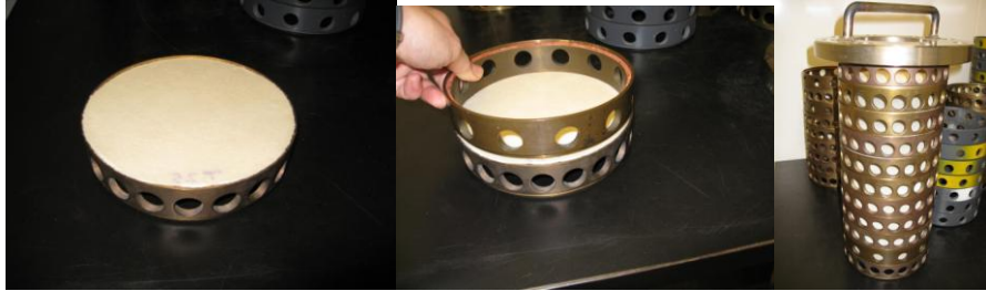
Figure 25: These are the drying components. On the left, place the disc to the holed copper (or PVC) rings; on the middle, place another drying ring on top of the handsheet; on the right, the handled stainless slab is the weight put on top of the drying ring stack during drying.
