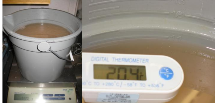
Figure 10: On the left, the disintegrated pulp has been diluted to 10 kg. Remember to measure sample amounts in weight, as volume is temperature dependent. On the right, the graduations are on the inside wall, 10 kg is at 11 L mark. This inaccuracy would cause serious problems in the following tests.
