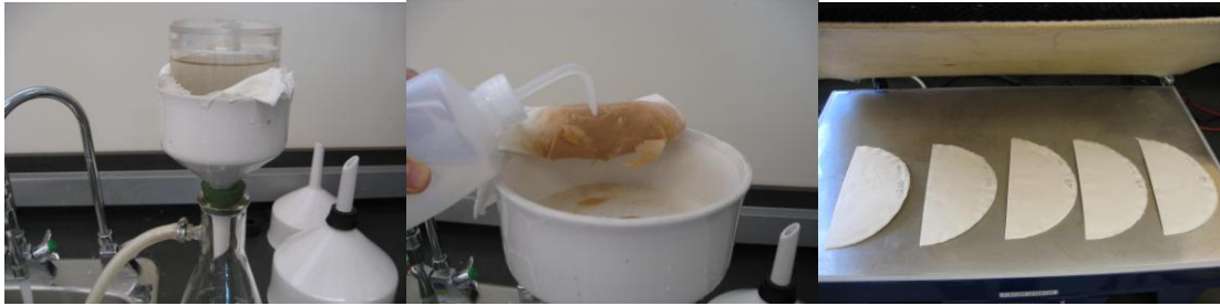
Figure 32: Procedure for fiber collection and drying. On the left, water removal is accelerated by using vacuum flask; in the middle, wash fibers to tared filter paper in funnel; on the right, dry the pulp pads in speed dryer.
