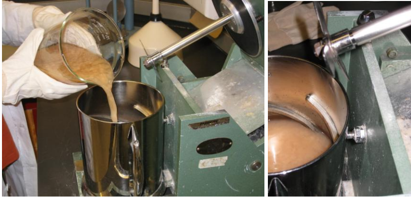
Figure 7: On the left, the heated pulp being poured into disintegrator apparatus; on the right, the vessel must touch the sensor stub in order for the disintegrator to operate.
