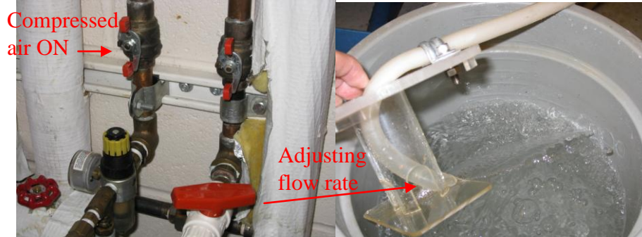
Figure 30: On the left, valves for compressed air and water; on the right, verifying the flow rate with a graduated bucket.
