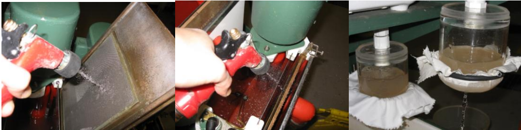
Figure 31: Collection of fibers. On the left, shower the screen to wash fibers off; in the middle, shower the vessel to wash out all of the fibers to sample cups; on the right, collecting fibers into sample cups.
