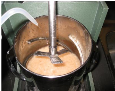
Figure 9: Pulp suspension after 7500 revolutions in the disintegrator. Squirt bottle is used to wash fibres off shaft and propeller.
