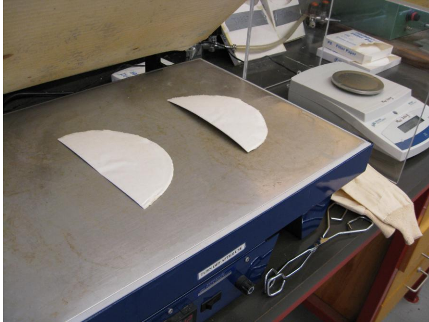
Figure 4: Semi-circle pulp pads being dried at speed dryer for consistency determination.
