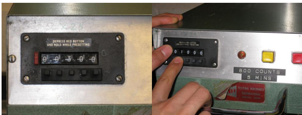
Figure 8: On the left, the button pad on the disintegrator; on the right, depress and hold the red button then push the black buttons to reset the revolution counts, which is required before you can disintegrate. Note: Each count equals 25 revolutions.
