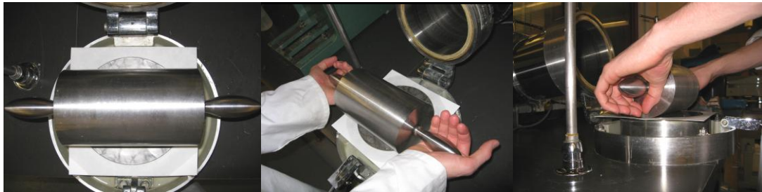
Figure 20: On the left, the couching pin is gently placed at the middle of couching disc; in the middle, rolling couching pin with palms up; or, on the right, rolling couching pin with circles formed by thumb and index fingers.
