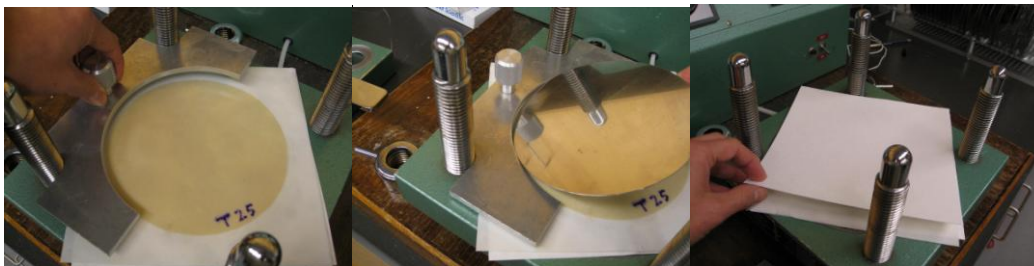
Figure 23: On the left, centering the handsheet; in the middle, place the pressing disc with an angle on top handsheet then drop it gently; on the right, place a new blotter on top of pressing disc.
