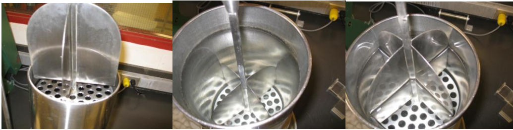
Figure 18: On the left, insert the plunger into the cylinder slowly; on the middle, the lower position of the plunger; on the right, the higher position of plunger.
